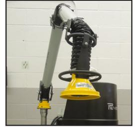
The Dust Extraction Swing Arm safely removes airborne dusts, gases and smoke emitted during the manufacturing process. These assemblies are fully mobile and retractable mounted onto a pivot arm extension. It also features a spring-loaded arm with an adjustable tensioner guarantees positive placement once fixed into the position of your choosing.
