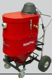
Ruwac's SumpPro Wet Vacuum Series is engineered to vacuum and pump at the same time. Emptying is as easy as flipping a switch. Our pump removes liquids at 38 gallons per minute, and each vacuum features various collection capacities. The compression cast composite housing will never dent or rust. The float assembly monitors liquid intake thus, eliminating the chance for overflow.
